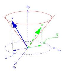
When  $x \succeq_{\mathcal{Q}} 0$ ,  $s \succeq_{\mathcal{Q}} 0$  are orthogonal both must be on the boundary in such a way that their projection on the  $x_1, \ldots, x_n$  plane is collinear
